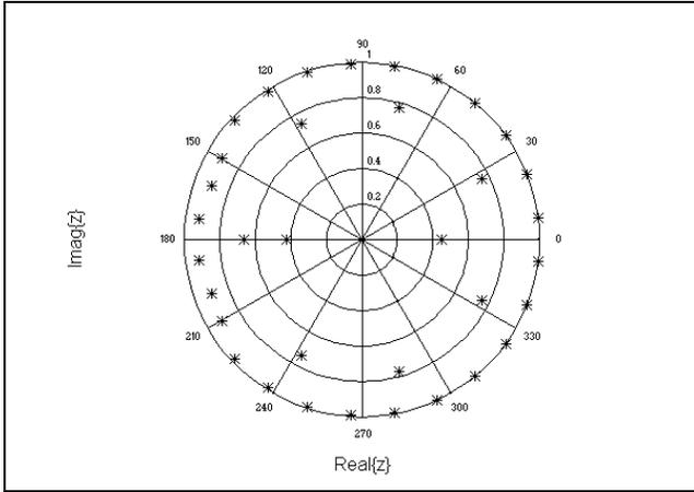
**Figure 3: LSMYWE AR Model Pole Locations**
